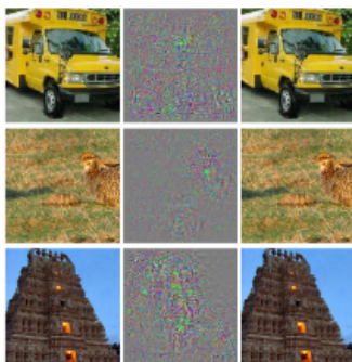
Figure 2: This image has been taken from [Sze+13, p. 6] and shows adversarial examples for AlexNet [KSH12]. The left column shows the true training images. The middle column shows a magnified version of the difference between the original image and the adversarial example. The right column shows the adversarial example corresponding to the true input which is misclassified.
