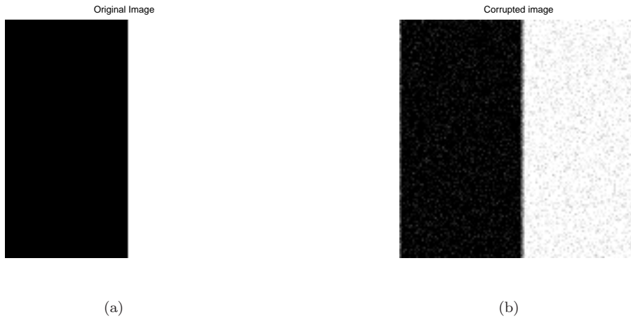
FIG. 6.9. (a) Original image that is black on its left and white on its right side. (b) Image corrupted by a blur operator with averaging kernel supported on 3 \times 3 pixels and uniform values 1/9 and additive white Gaussian noise with variance 20.
